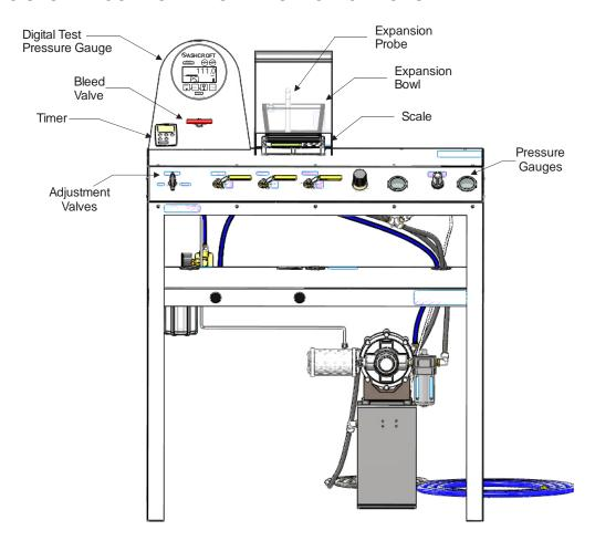
Figure 2- 1 Digital GTC Test Console
