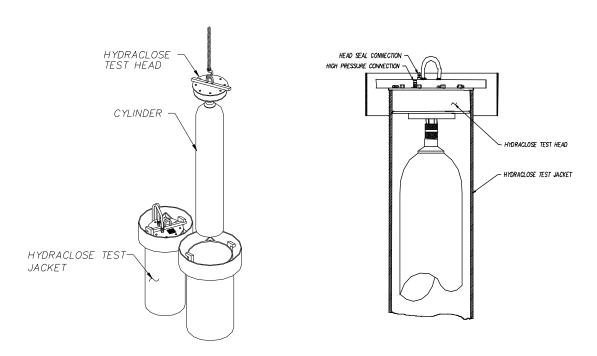
Figure 5 - 1 Cylinder/Test Head Installation
