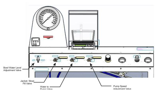
Figure 5 - 5 GTC Control Panel
