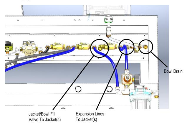
Figure 4-3 Digital and Analog GTC Console Plumbing
