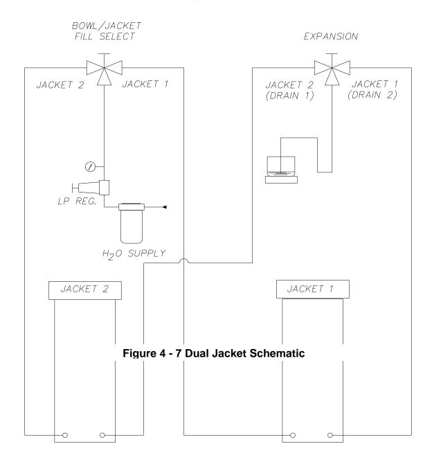
When utilizing both Jackets, it is advisable to completely disengage the Test Head on the Jacket that is not testing. This is so the Safety Interlock, of the non-testing Jacket, is not engaged while the other Jacket is testing.
