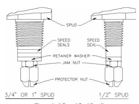
Figure 4 - 6 Speed Seal Details
