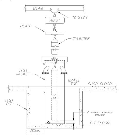
Figure 4 - 1 Example Hydrostatic Test Pit
