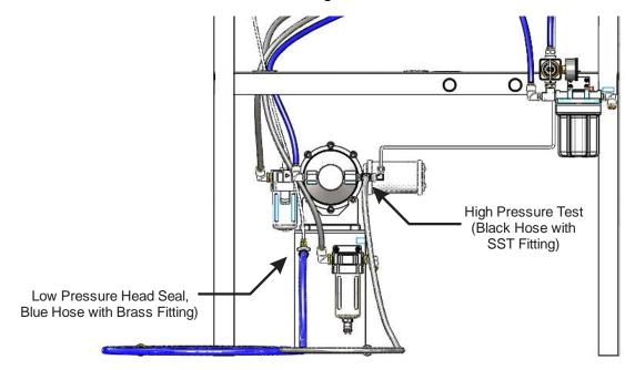
Figure 5 – 2 Hose Connections
