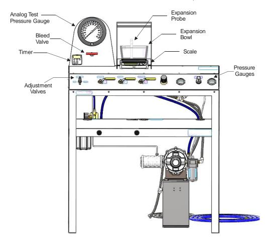
**Figure 2-2 Analog GTC Test Console**
