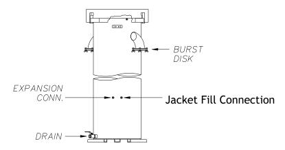
Figure 4 - 4 Hydrostatic Test Jacket
