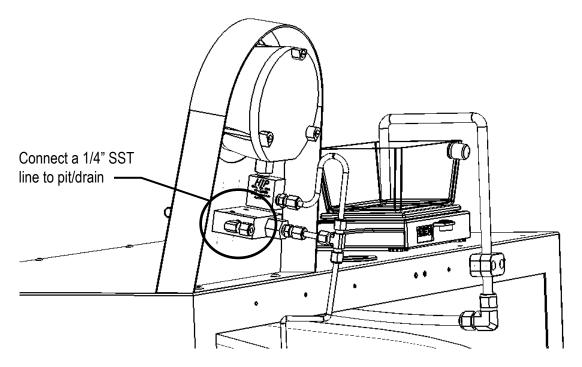
Figure 4-3b.1 Digital GTC Console Plumbing
