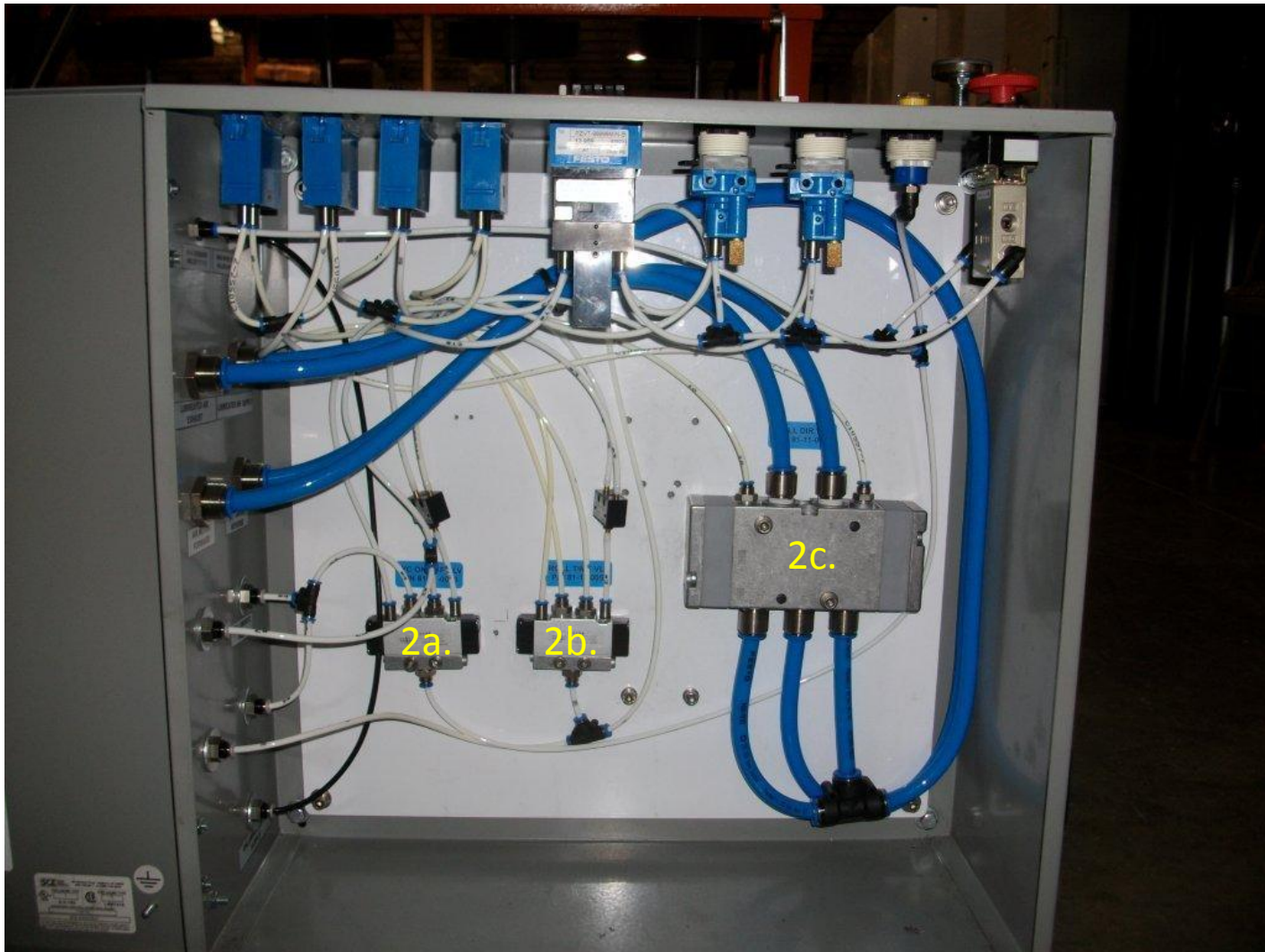
2a. Cycle Start Stop 5 way valve 2b. Roll Time 5 way valve 2c. Roll Direction 5 way valve
